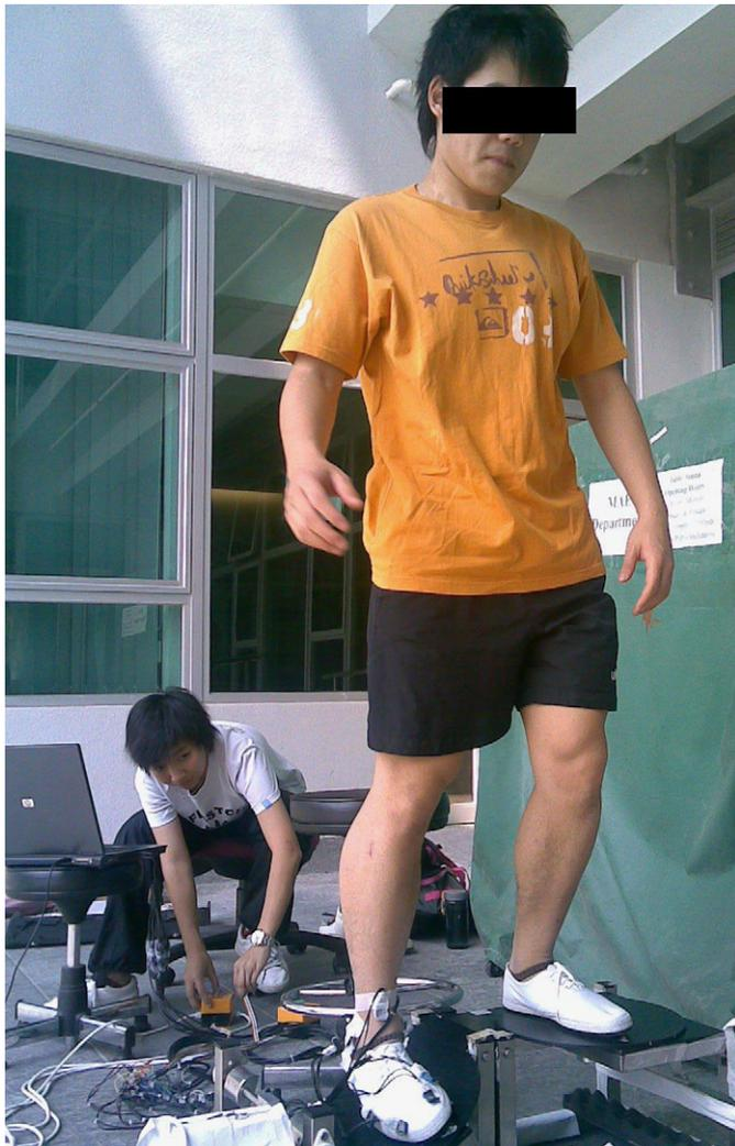
Fig. 2. . Experimental setup for data collection on ankle simulated sprain.
