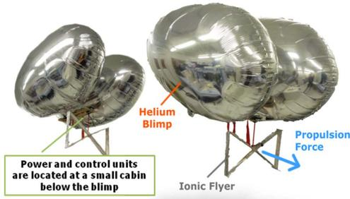
Fig. 11. Prototype of the Ionic Propulsion Blimp.
